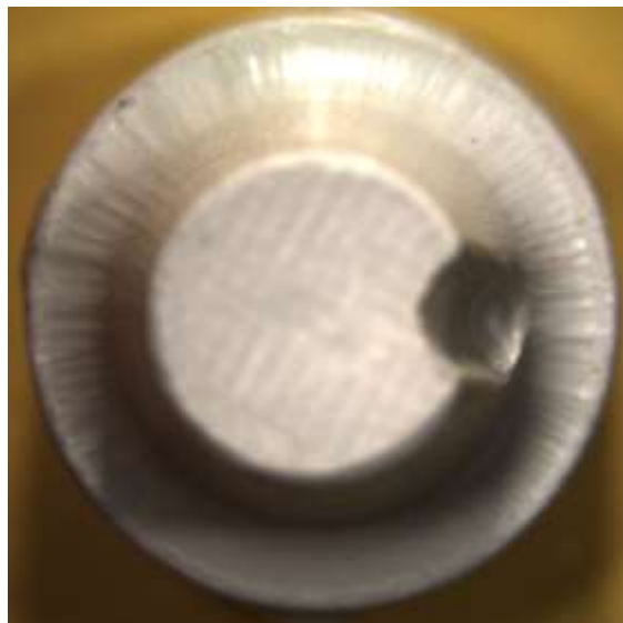
Fig. 1: Master die with anti-rotation groove.
