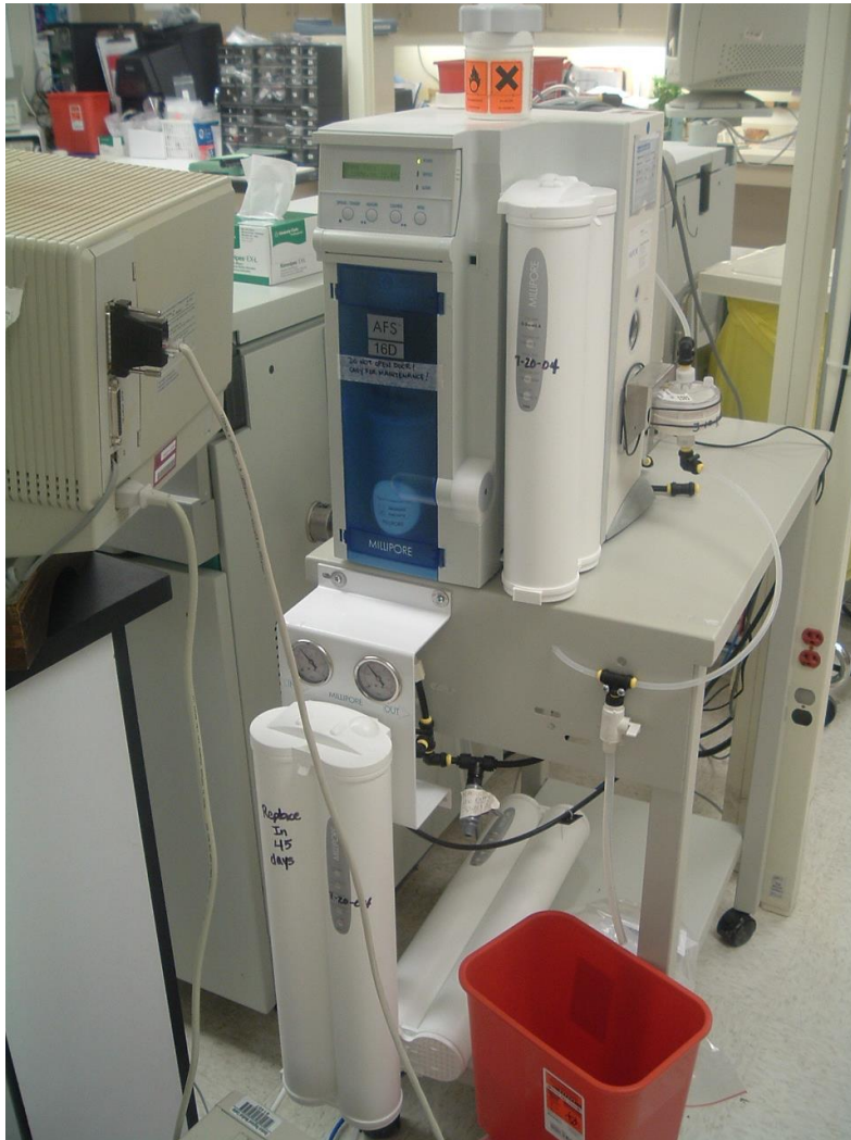
Water filtration system for Automated chemistry analyzer.
