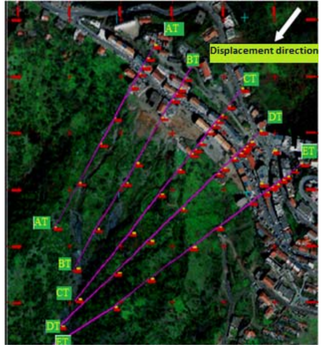
Fig. 2 Satellite photos with the topography monitoring sections
